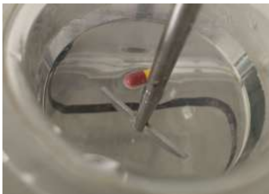
Fig. 2: Dissolution of capsules containing solid dispersion of telmisartan and hydrotropic agent (sodium tartrate)
